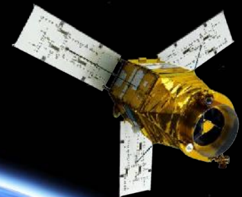
KOMPSAT-3 Design lifetime : 4 years 2012.5.18 - 0.7 m EO Payload LTAN : 13:30
